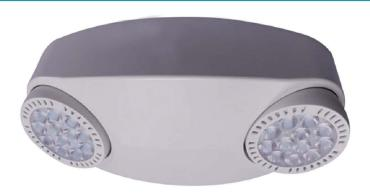
The HPEM series is a thermoplastic emergency lighting unit with built in lithium iron phosphate battery that provides 90 min of illumination during an emergency. This adjustable lamp head provides up to 100 ft center-to-center spacing with a 3-ft path of egress at 7.5 ft mounting height. This light features a low profile, contemporary design with LED economy and dependability. Adjustable heads ensure any application is lit. Standard with 1,162 lumen output (581 per head x 2)
