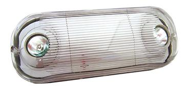
The RMR-16 series thermoplastic emergency light combines a low-profile, contemporary appearance with durability and dependability. Constructed of an injection-molded, SVA flame rated, high-impact, UV-stabilized thermoplastic housing, it is ideal for high-vandalism, wet locations and is resistant to corrosive atmospheres and non-hazardous dust environments. It is standard with 3.3W LEDs that provide a minimum of 90mins of illumination during an emergency.
