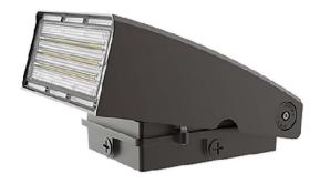
This wattage and Kelvin selectable full cutoff adjustable wall pack is a contemporary, commercial grade area light fixture. It features a heavy-duty, spring-loaded hinge. This light has a durable die cast aluminum housing and a polycarbonate lens. This fixture is standard with photocell installed. Its housing serves as a junction box for easy install and wiring.
