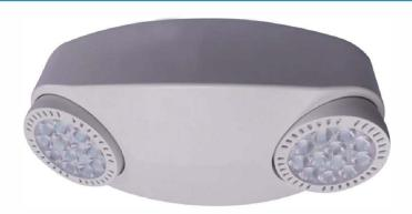
The HPEM series is a thermoplastic emergency lighting unit with built in lithium iron phosphate battery that provides 90 min of illumination during an emergency. This adustable lamp head provides up to 100 ft center-to-center spacing with a 3-ft path of egress at 7.5 ft mounting height. This light features a low profile, contemporary design with LED economy and dependability. Adjustable heads ensure any application is lit. Standard with 1,162 lumen output (581 per head x 2)
