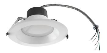
The 4", 6" and 8" Architectural Recessed Downlight Retrofit solution has an integrated LED power supply and thermal management system combined in a single compact unit designed to fit most standard 4", 6" and 8" openings. Also works in new construction applications. It is wattage and kelvin selectable to fit most needs and wet location rated.
