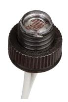
Light-sensitive photocell switches direct fixtures to turn off when ambient light is present, and switches them on when ambient light is absent. Ideal for use with outdoor light fixtures requiring photoelectric automation. Rain-tight for outdoor use. Preset time delay prevents unintended switching from flashes due to headlights, lightning and other temporary lighting sources.
